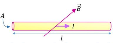
As force acting on one electron is  $f = ev_d B \sin \theta$  where  $v_d$  is the drift velocity of electrons.
