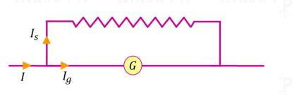
shunt resistance R in parallel with it which is obtained as
