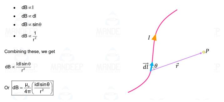
Where  $\theta$  is the angle between r and dl and  $\mu_o = 4\pi \times 10^{-7} \text{TmA}^{-1}$  is called **magnetic permeability of free** space.
