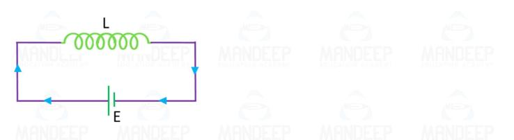
Consider an inductor of inductance L connected to a voltage source E as shown in figure above. Let current at any instant be I.
